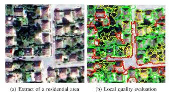
Fig. 12. Visualisation of local quality estimates. Yellow segments correspond to over-segmentation, red segments correspond to under-segmentation and green segments correspond to well isolated segments.
