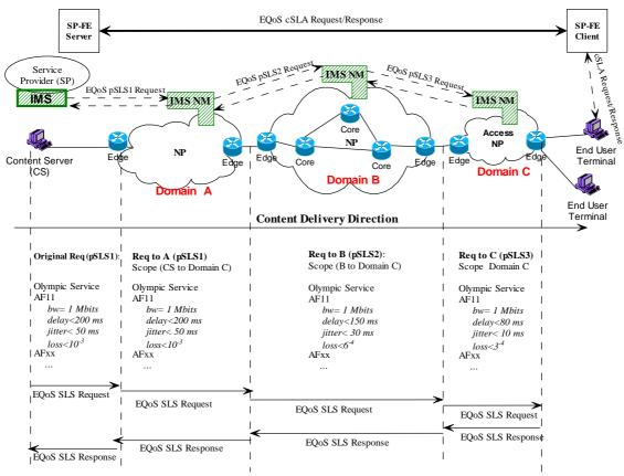
Figure 5: Service Level Specification Signaling Protocol.
