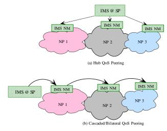
IMS NM : IMS Network Manager IMS @ SP : IMS at Service Provider NP : Network Provider
