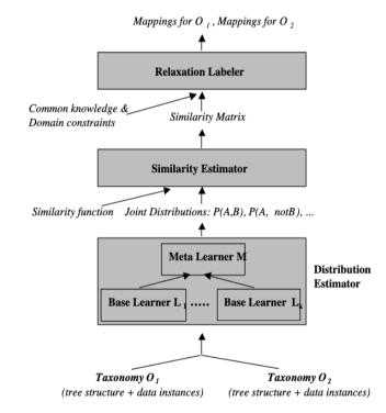
Fig. 2. The GLUE Architecture
