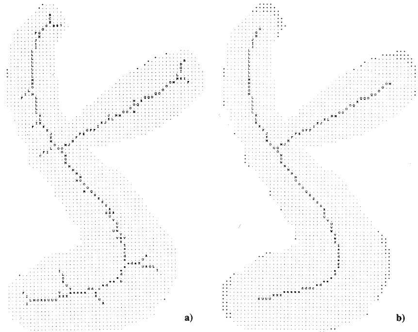
Fig. 3. The (3,4)-weighted skeleton of a pattern before pruning (a) and after pruning (b). The pixels of the input pattern which are not recovered by applying to the skeleton the reverse distance transformation are indicated by "+".
