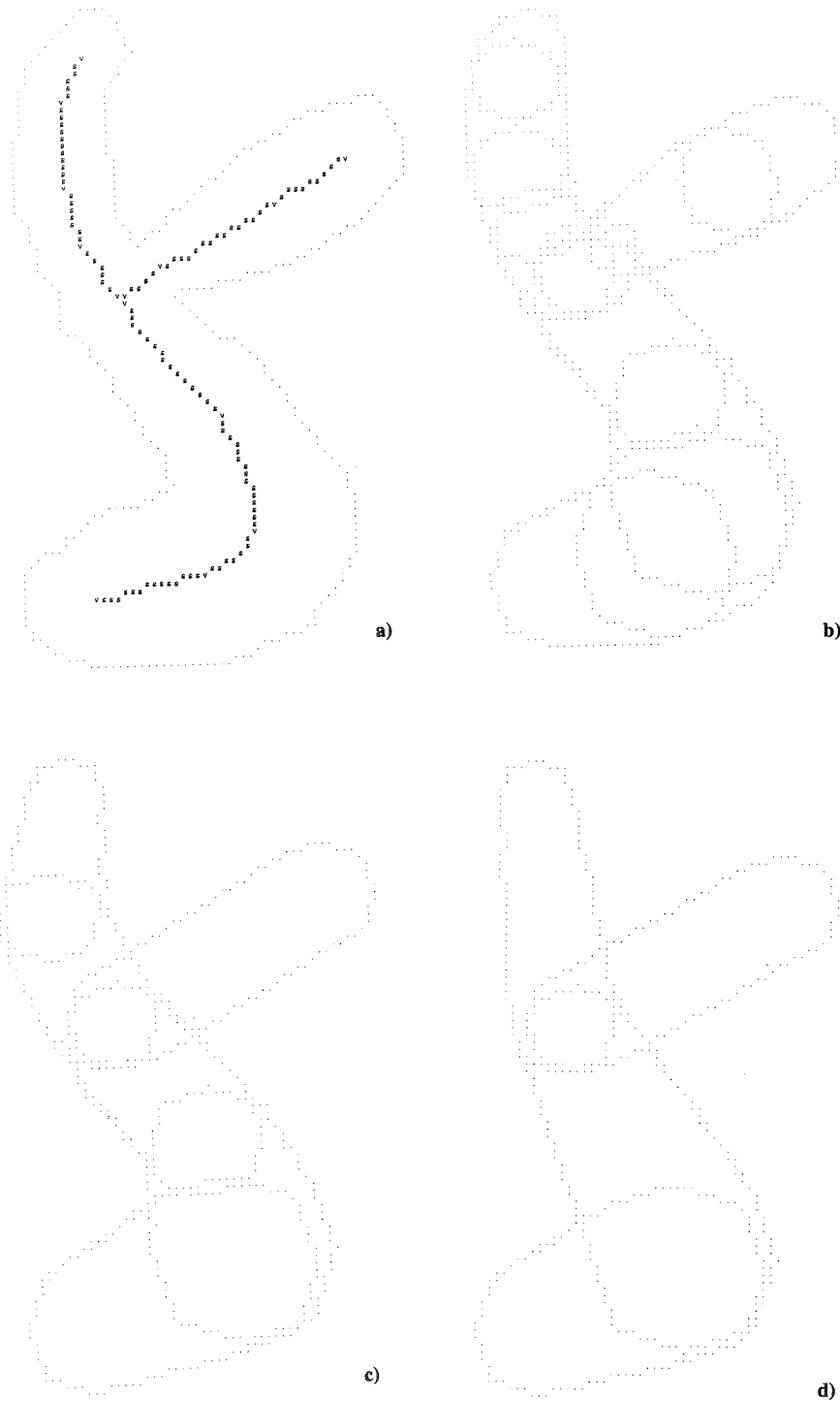
Fig. 4. Letter V denotes the vertices found during the polygonal approximation of the skeleton with threshold \theta = 1.5 (a); decomposition into elementary regions, corresponding to \theta = 1.5 (b), \theta = 4 (c), and \theta = 8 (d).
