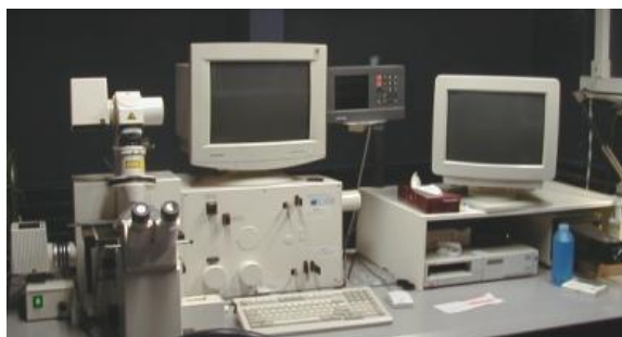
FIG. 2.17 – Microscope Zeiss Axiovert 410
