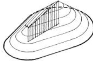
Fig. 4. A three-dimensional static alternative to the two-dimensional kinetic view of the process. (The MAF is the ridge formed where the union of cones on the input contour intersect each other.)
