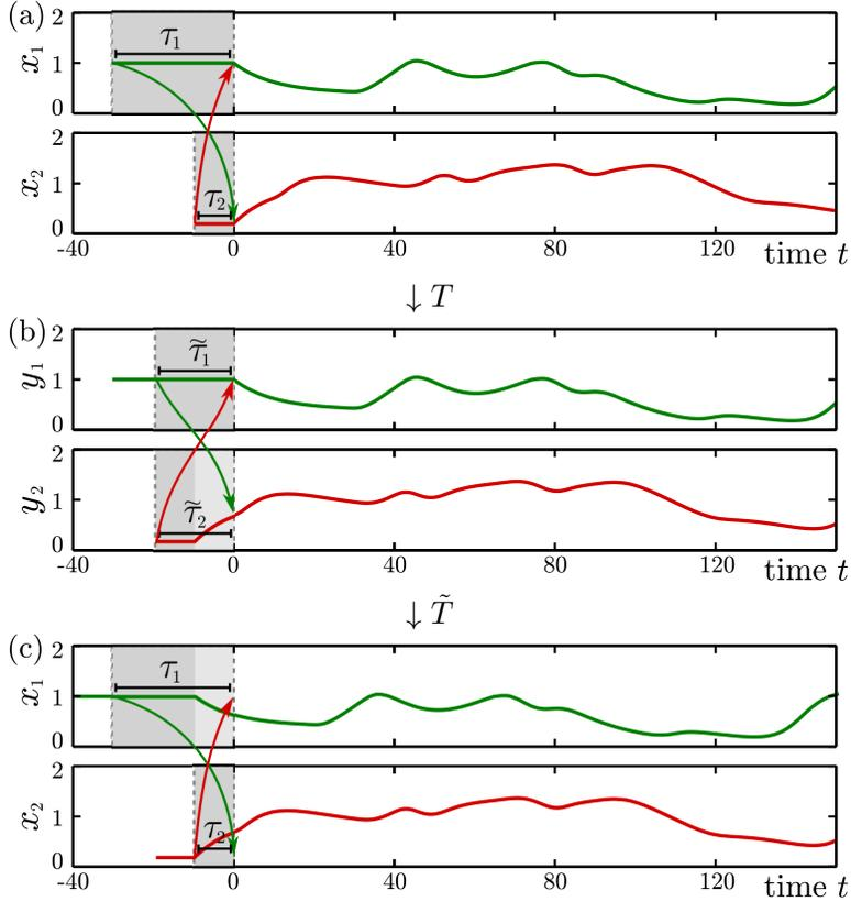
**Figure 2.** *CT-Transformation for a pair of bidirectionally coupled Mackey-Glass systems [26], cf. Fig. 1. Plot (a) shows the original solution  $\mathbf{x}(t) = (x_1(t), x_2(t))$  of (2.1). Plot (b) shows the transformed solution  $\mathbf{y}(t) = (y_1(t), y_2(t))$  of (2.2), which is shifted to the left by amounts  $\eta_1 = 0$  and  $\eta_2 = 10$ . Plot (c) shows the solution  $\mathbf{x}(t + \eta_1)$  obtained after a reverse transformation of  $\mathbf{y}(t)$  [see §4 for details].*
