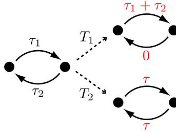
**Figure 1.** Two simple examples of CT-Transformations for a ring of two delay-coupled systems. The transformation  $T_1$  reduces the number of delays from two to one and  $T_2$  reveals a hidden symmetry in the system by adjusting the two delays to the same value  $\tau = (\tau_1 + \tau_2)/2$ .
