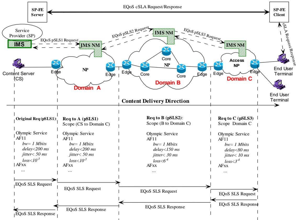
Figure 5: Service Level Specification Signaling Protocol.
