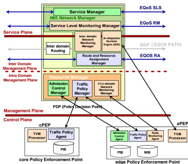
Figure 4: High Level Functional Architecture.
